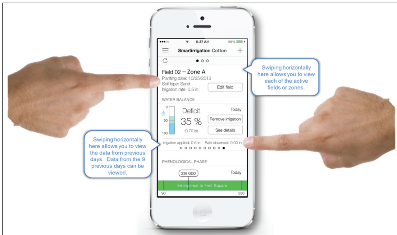
Figure 2. Screenshot of the SmartIrrigation Cotton App indicating how users can view data from multiple fields or zones as well as from up to nine previous days. The root zone soil water deficit is displayed both graphically and numerically in the center of the screen.
